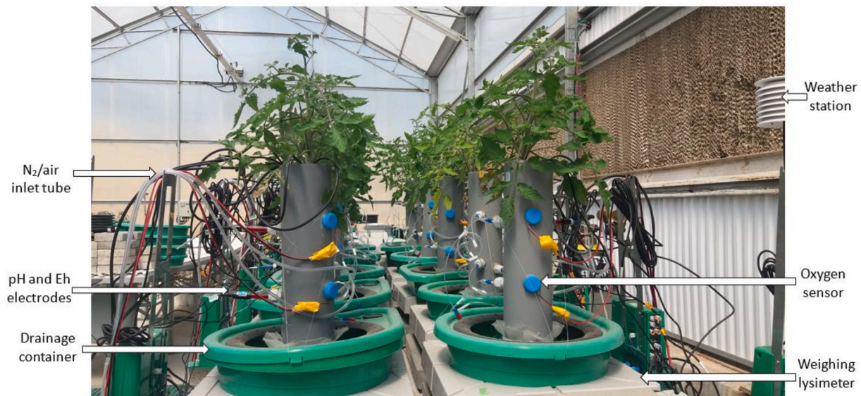
Fig. 1. Experimental platform used to impose N_2 -induced hypoxia under non-flooded conditions while continuously monitoring whole-plant and rhizosphere responses in Exp. 1 and Exp. 2. Tomato plants were grown in PVC soil columns mounted on weighing lysimeters (PlantArray 3.0) positioned above drainage containers. N_2 -induced hypoxia or aerated control conditions were imposed by continuous delivery of N_2 or air through an inlet tube inserted into the soil column. Rhizosphere pH and redox potential (Eh) were monitored using electrodes inserted through dedicated side ports, and soil O_2 was measured using an oxygen sensor installed in the column wall. Environmental conditions were recorded by the greenhouse weather station. The system enabled continuous gravimetric, environmental, and rhizosphere monitoring throughout the experiment.
