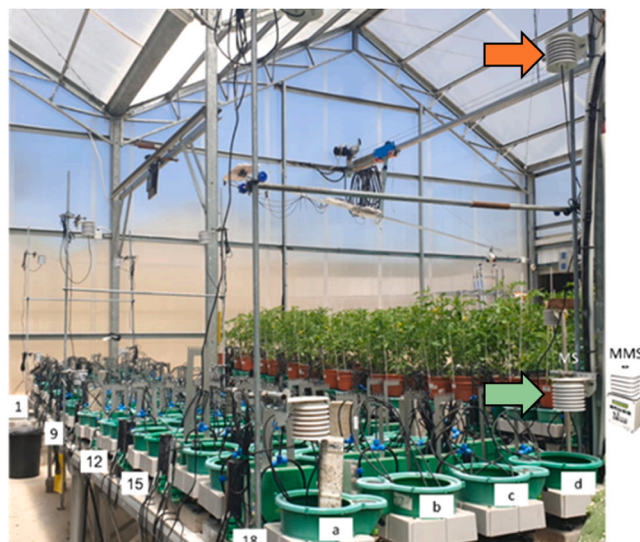
Fig. 1. Experimental greenhouse bench equipped with a gravimetric evaporation platform and spatially distributed meteorological sensors. The experimental bench (7 m × 1.2 m × 0.9 m) was arranged in 18 columns (1–18) and 4 rows (a–d) and included 72 load-cell lysimeters (Plant-DiTech, Israel). Sixty-two lysimeters were mounted with evaporation pans (22 cm diameter, 5 cm depth), automatically refilled daily at 04:00. Ten additional lysimeters held constant weights for drift correction. Twelve meteorological stations (MS), measuring temperature, relative humidity, and barometric pressure, were installed at six positions: (1,a), (1,d), (9,a), (9,d), (18,a), and (18,d), each with two vertical heights: Z_0 (30 cm above pan level, marked with green arrow) and Z_1 (1.5 m, marked with orange arrow). The main meteorological mast (MMS), located near (18, d), recorded additional environmental parameters.
