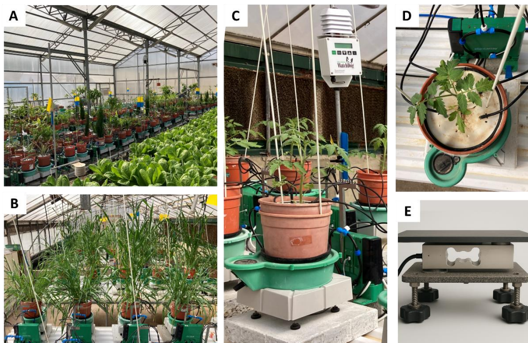
Figure 1: Configuration of load cell lysimeter system and greenhouse. (A) Main greenhouse containing various crops monitored using the PlantArray phenotyping platform. (B) Secondary greenhouse with wheat plants monitored using the same system. (C) Image of a single PlantArray unit, showing the load-cell lysimeter, double-pot setup, “personalize” controller collecting data and controlling each pot irrigation, and the central weather station used for continuous environmental monitoring. (D) Top view of a pot showing the sealed soil surface cover, designed to isolate plant transpiration from soil evaporation. (E) Photorealistic illustration of a single lysimeter unit. It includes a temperature-compensated load cell that converts mechanical force into an electrical signal, directly connected to the controller. The cell is mounted between two steel platforms to ensure stable weight measurement. As shown in (C), the lysimeter is typically covered with a polystyrene block and a thermal-isolated lid.
