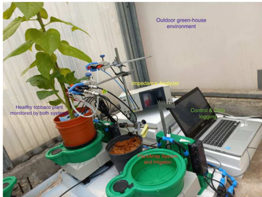
Figure 1 Tobacco plant monitored by both the impedance system, and the PlantArray gravimetric system set up at a greenhouse in Tel- Aviv.
